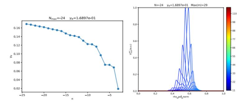
Normalised growth rate scaling with toroidal mode number (left) and radial velocity component of the most unstable mode (right) are shown for the CDBM equilibrium with fast ion pressure included.
