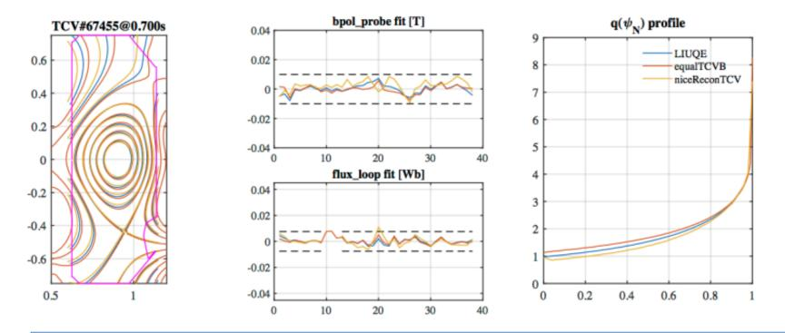
Good agreement is found between the several codes (LIUQE – the in-house tool at TCV, EQUAL and NICE). Comparison of flux contours, magnetic probe and flux loop reconstruction errors and obtained |q| profiles for the codes LIUQE, EQUAL and NICE using data from TCV discharge 67455 at t = 0.7s. Black dashed lines indicate the absolute error for the different signals
